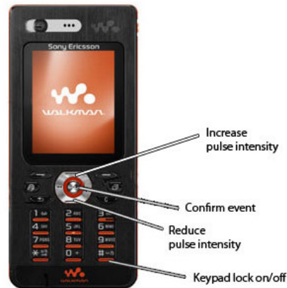
Fig. 3: Second prototype, with keyboard configuration
