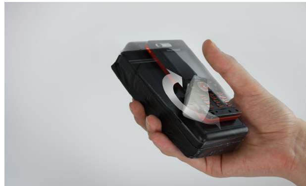
Fig. 1: Prototype. Sony-Ericsson W880i mobile phone, mounted on weight-actuated box.
