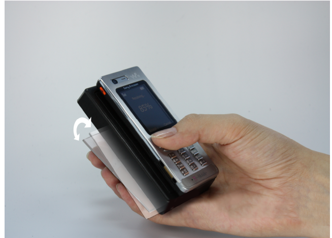
Fig. 1: Prototype, consisting of a mobile phone, mounted to a shape-actuated box.
