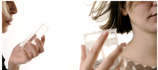
Figure 3: Whispering prototype, whispering telecommunication through airstream sensing and actuation on front side.
