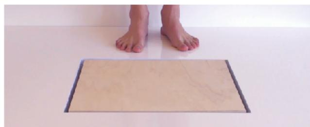
Figure 4. The supporting points of the upper frame can be set to different materials and therefore users can explore three degrees of rigidity
